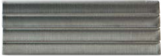
Range 2 cuts on 6 mm (1/4") mild steel
