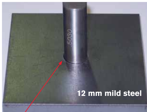
12 mm hole with True Hole technology cut with HPRXD® Plasma
